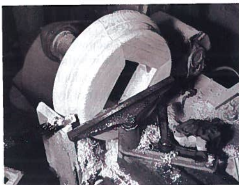
In open-face turning the work is supported on just one side of the lathe.
