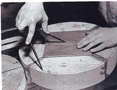
Accurately marking the center and circumference of a base blank keeps it balanced.
